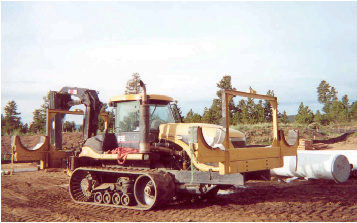
(Challenger Pipe Carrier shown with optional Hiab knuckleboom crane)
