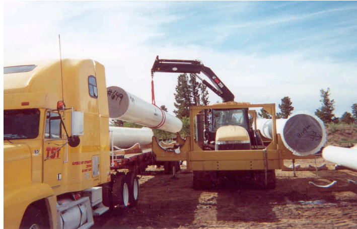
(Challenger Pipe Carrier shown with optional Hiab knuckleboom crane)
