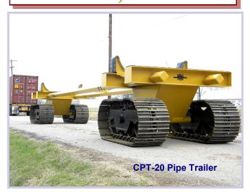
These Challenger Services trailers utilize the Steel Track design providing more flotation and resistance to rock and stump damage than rubber tires.
