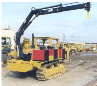
Caterpillar D6E Tractor—Shown with Hiab 060 Knuckleboom
