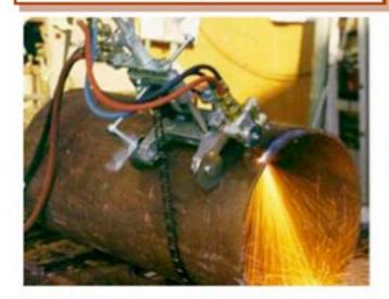
Koike Aronson Portable Cutting Solutions Pipe Cutting Machines.
